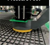
CAMTRON unique dust free pressure foot design. This revolutionary design helps keep your workshop clean and help stabilizing the material.
